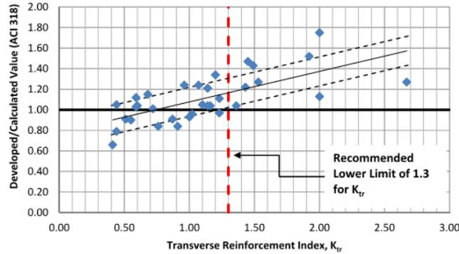
Figure 3-3 Developed-to-calculated stress values versus transverse reinforcement index,  $K_{tr}$  (based on data from Sellem et al., 2009).
